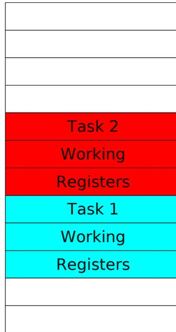
As you can see, the register contents for Task2 are stacked on top of Task1 (hence the term 'Stack'). Now suppose Task3 is completed, and the microprocessor wished to return to its previous job. It simply pulls from the stack the register contents for the job that was interrupted last and carries on (back to (2)). When this job is complete, it again returns to the previous state by pulling from the stack the previous state of its registers.
